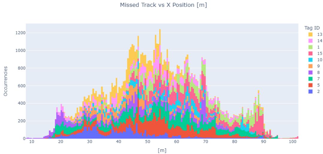
Figure 4.50: Histogram representing all positions along the X-axis of the sensors of players that either have not been detected by ByteTrack, or have no tracklet assigned, for the complete video ( \sim 22 minutes) under investigation. Different colors refer to positions of different players, which are uniquely identified by their sensor ID ( tag_id ).
