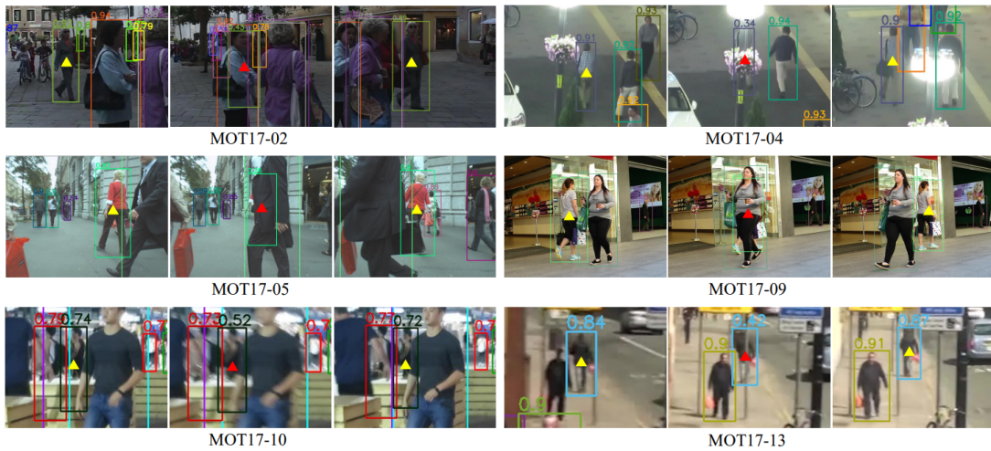
Figure 2.15: Visualization results of ByteTrack coming from MOT17 validation set. Note as also in case of occlusion or motion blur the algorithm behaves correctly. Yellow triangles denotes high score detection boxes, whereas red triangles low score and boxes with the same color refer to a unique trajectory. (image from [2]).
