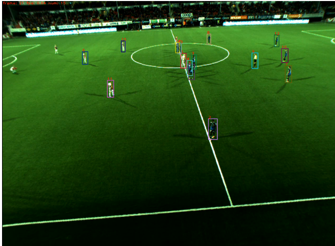
(a) A sample frame from the video that ByteTrack has returned as output. The players that are detected are assigned with a colored bounding box, above which there is a number that uniquely identifies it.
