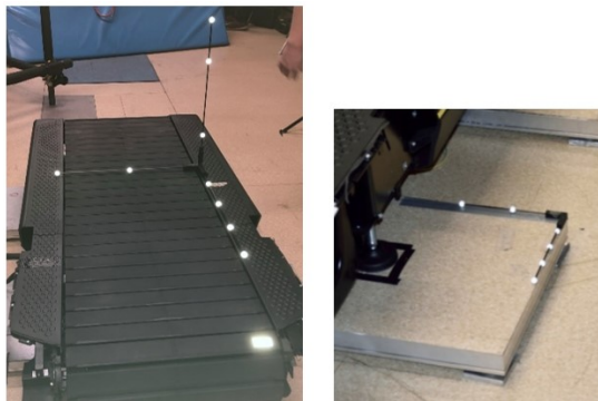
Figure 3.4: Triads on the treadmill representing the absolute reference frame and the smaller L-frame to locate the force platform.
