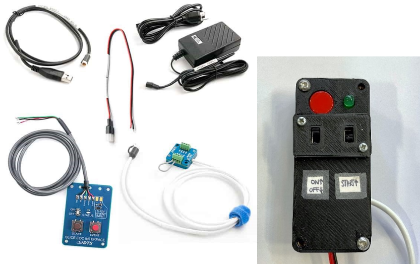
Figure 3.12: SLICE NANO Base Cable Kit on the left: it includes the End-of-Chain (OEC) terminal, start-event switch, USB communication cable and power supply. The custom case on the right.
