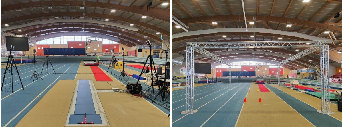
Figure 6.17: New instrumentation at the Palaindoor of Padua: Force platforms (left) and framework (right).
