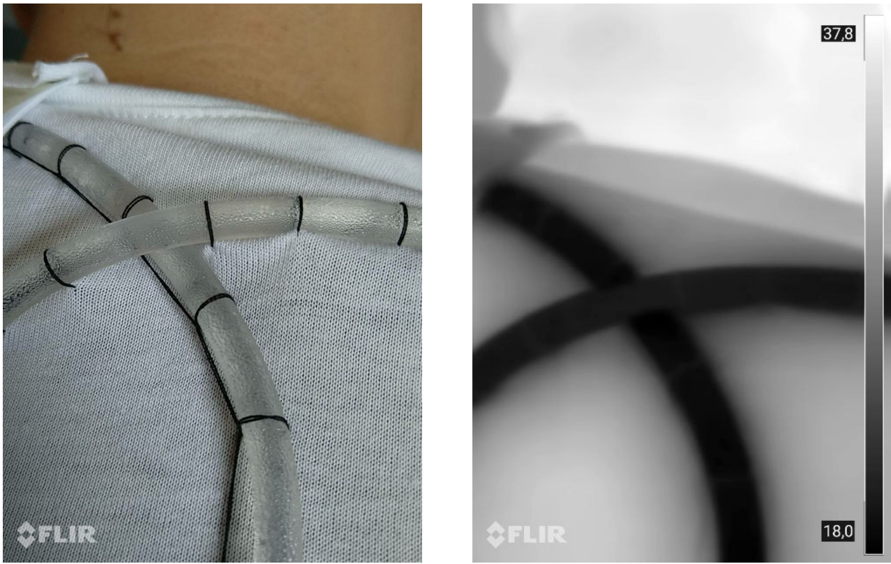
Figure 2.4: Detail of the stitched tube in the final garment; black thread is used for contrast
