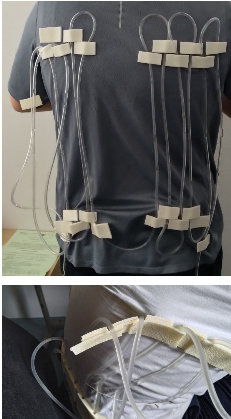
Figure 2.2: Pictures of adhesive de-bonding due to condensation in early prototypes; peeling is noticeable as adhesives are most sensitive to that failure mode
