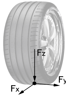
Figure 4.2: Forces acting on the tire-road contact point.
