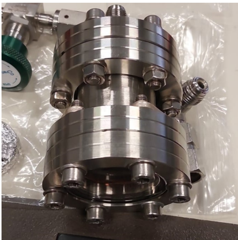
Figure 3.22 - Vacuum receptacle to transport the sample of Au (111) with deposited MoS 2 . In the picture the receptacle is not yet complete, missing its valve, seen in the top left-hand corner, to seal it once the vacuum has been pulled.
