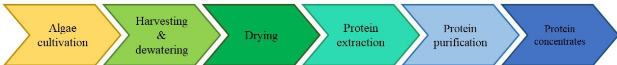
Figure 3.2.2 – Principal steps used in the production of algal protein concentrates (Kumar et al., 2022b).
