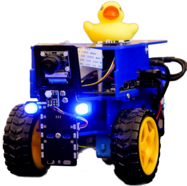
Figure 1.1: Duckiebot mobile robot used as a reference platform in this thesis, equipped with wheel encoders, IMU, and a monocular camera.
