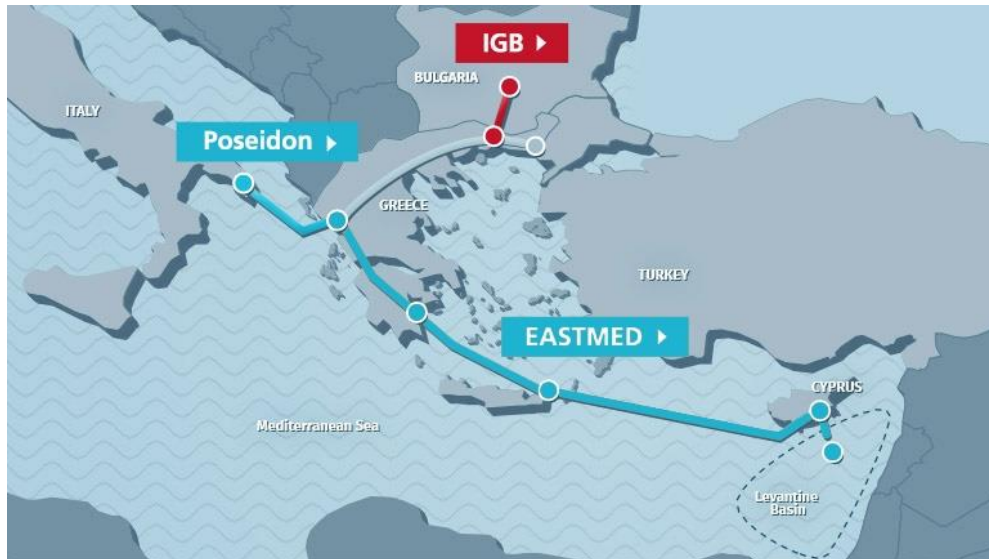
Figure 3.2.A-4: Map of the East-Med pipeline project. In light blue: the offshore sections of the pipelines; in grey: the onshore section of the Poseidon Pipeline; in Red: the interconnection with the IGB (source: Samaha 2019)
