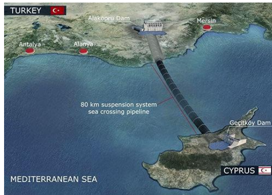
Figure 3.2.B-2: Water pipeline connecting Turkey and Cyprus. (Source: Daily Shabah)
