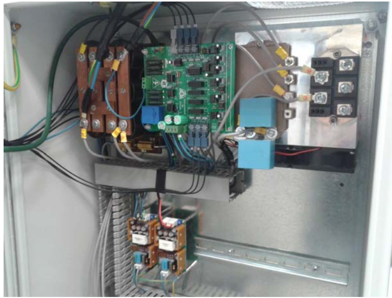
Figure 5.3: Inverter connected to the IPMSM
