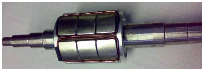
Figure 1.15: SPM rotor with ringed-poles [9]
