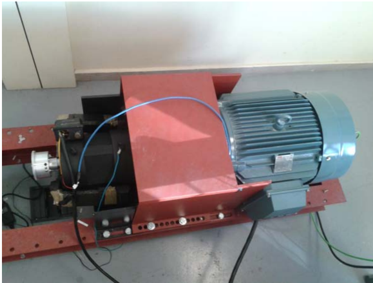
Figure 5.5: IPMSM coupled with the IM
