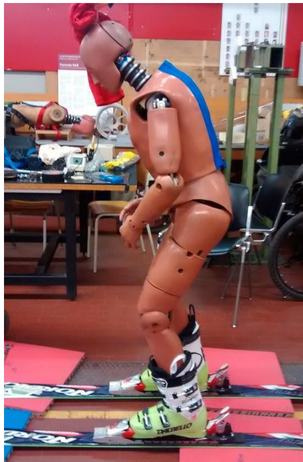
Figure 6-26: anthropomorphic dummy wearing skies
