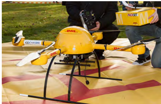
Figure 4.2: The UAV used by DHL to deliver a small parcel across the Rhine.
