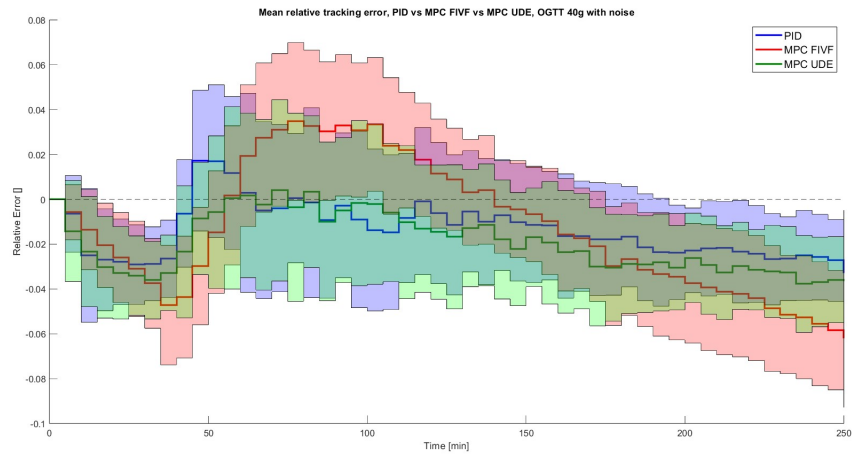
Figure 5.9: Comparison between PID, MPC FIVF and MPC UDE controllers on population, relative tracking error, ISO-IV clamp (OGTT 40g), measurement noise present.
