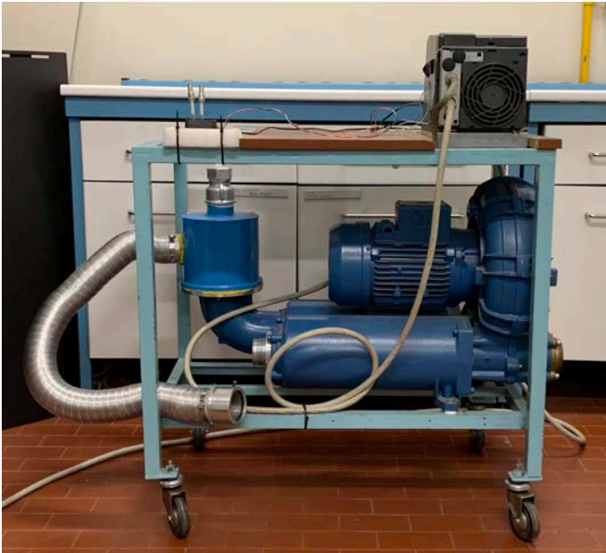
Figure 2.6: Blower with its inverter.
