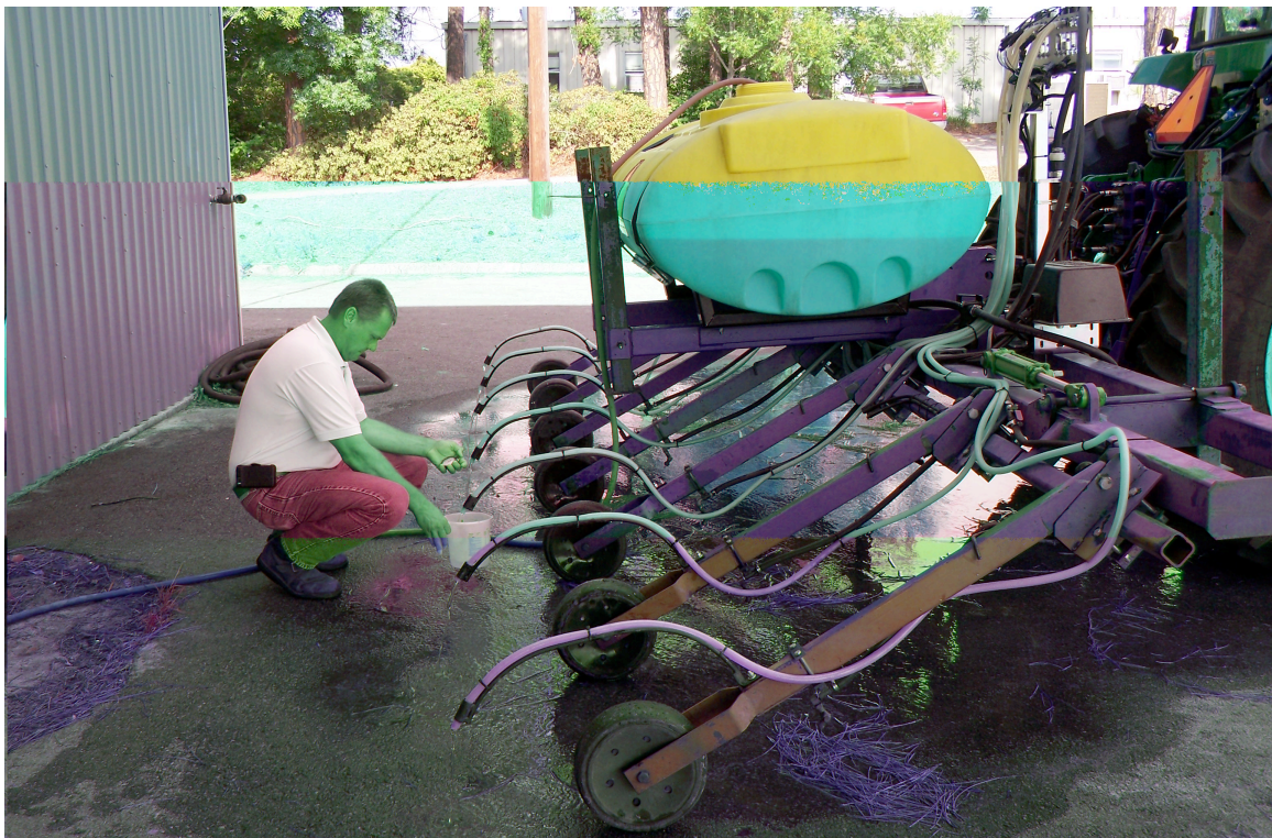
Figure 2.6 – Sprayer calibration; it occurred calculating a prescribed flow rate of water in order to estimate the corresponding real emitted flow
