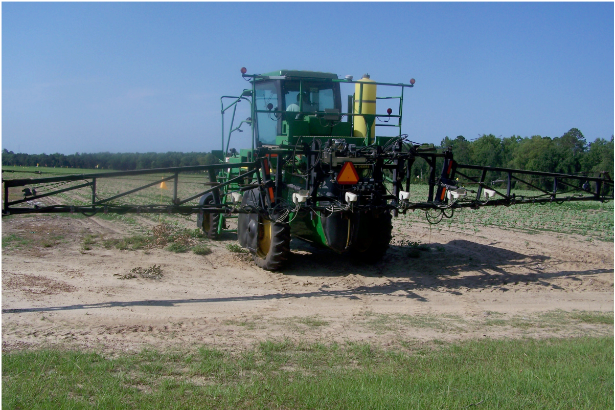
Figure 2.11 - John Deere High Boy sprayer equipped with GreenSeeker® sensors
