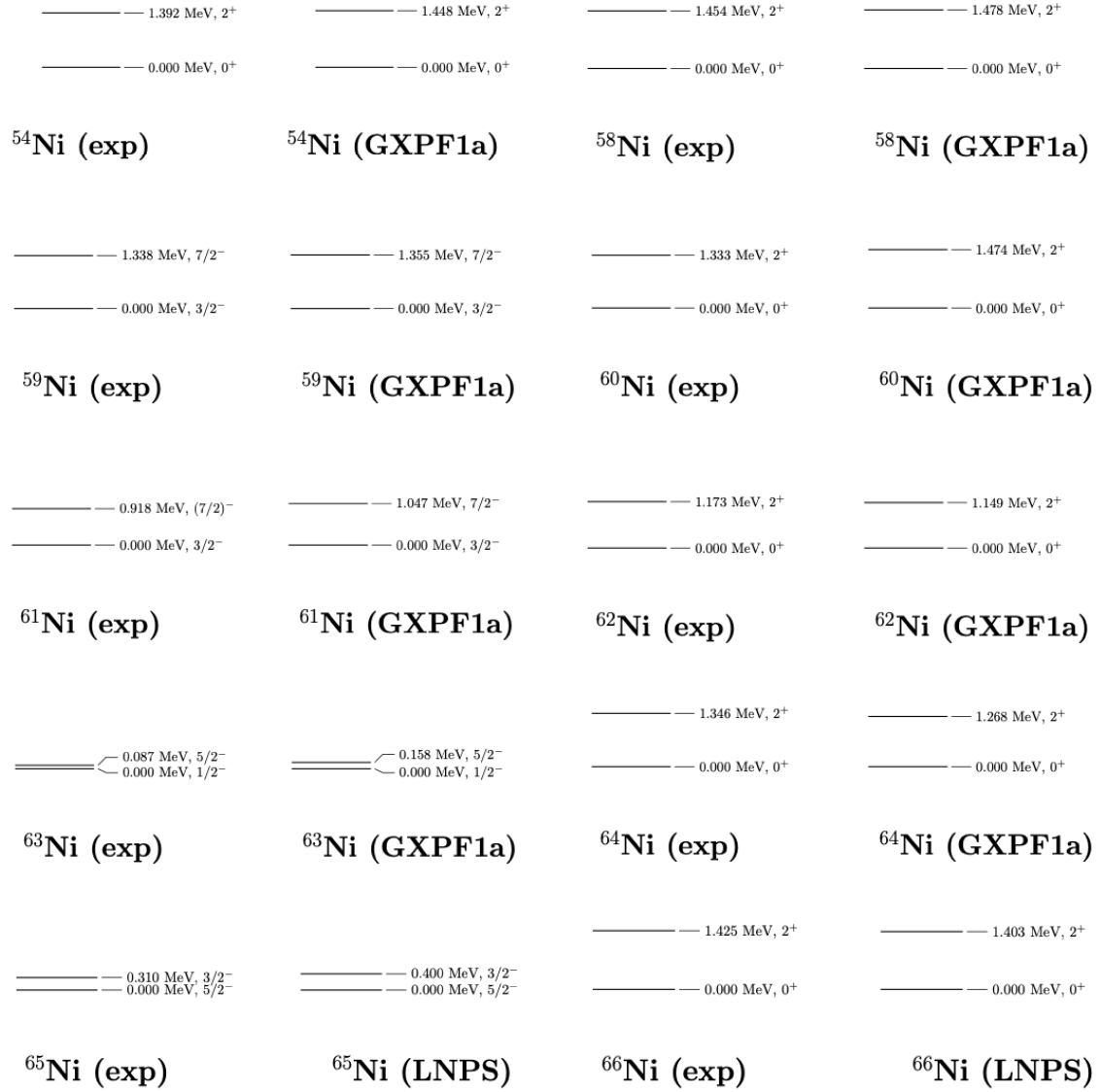
Figure A.7: Energy levels for the Ni isotopes calculated via the GXPF1a interaction [27] for ^{54-64}\text{Ni} isotopes and with the LNPS interaction [28] for ^{64-70}\text{Ni} ones; the results are then compared with the experimental ones [44].
