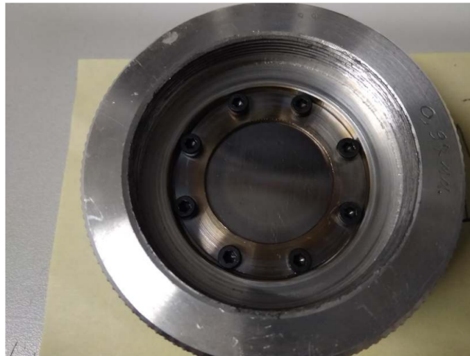
Figure 2.7: Picture showing the fresh nat3 target mounted on the target holder. The beamspot is visible in the middle of the target.
