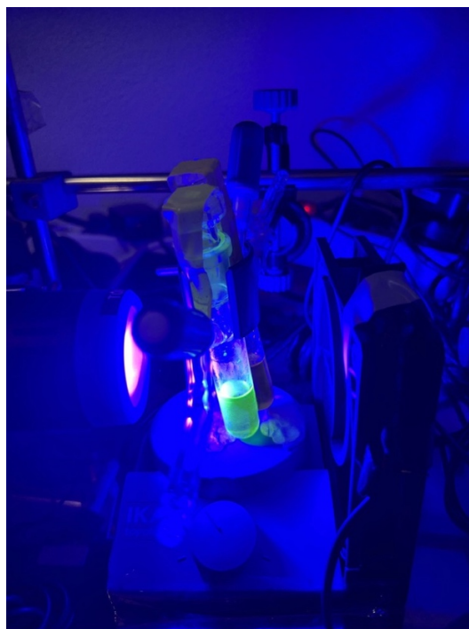
Figure 48. Photochemical setup for the Giese-type addition. The distance between the Schlenk and the Kessil lamp is 3 cm. The system is ventilated with a fan.
