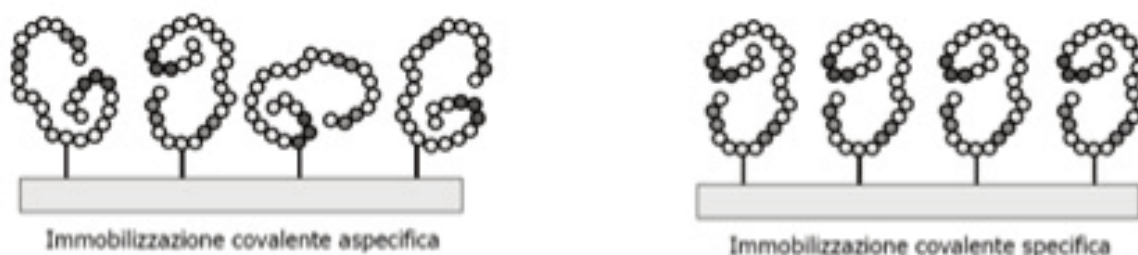
Figure 1.2: Covalent immobilization, non-specific (left) and specific (right).
