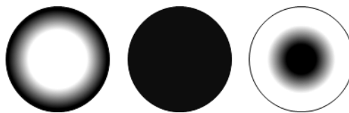
Figure 6.3 Drawing of the three cases, from the left: a coffee ring effect deposit, a perfectly homogeneous deposit and a reverse coffee ring deposit.
