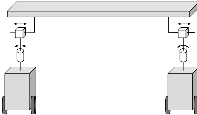
Figure 4.6: Joints connecting the robots with the transported object. On the bottom, two differential drive mobile robots serve as the base platform. Each robot is surmounted by a revolute joint and subsequently by a prismatic joint which is connected to the to-be-transported object.
