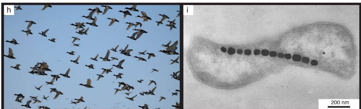
Figure 3: Macroscopic image of migrating birds, in (h), and TEM micrograph of a magnetotactic bacterium with magnetite nanoparticles arranged along the long axis of the cell, in (i). Adapted from [7].
