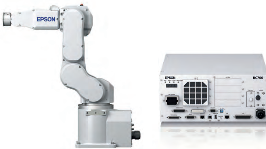
Figura 2.1: Modello Epson C4 e controller Epson RC700 [4].
