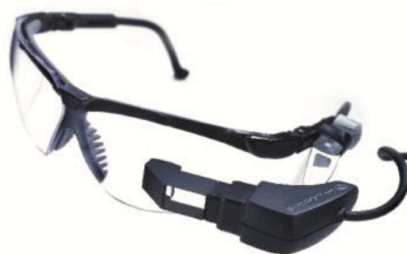
Figura 10: MicroOptical SV6 "display opaco monoculare" (Plouznikoff, 2005)
