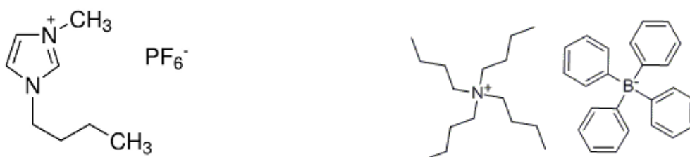
Fig.3.2 1-butyl-3-methylimidazolium hexafluorophosphate structure on the left, and tetra-n-butylammonium tetraphenylborate structure on the right.
