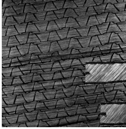
Figure 5.7: Example of CutMix augmentation for a missing stitch defect.
