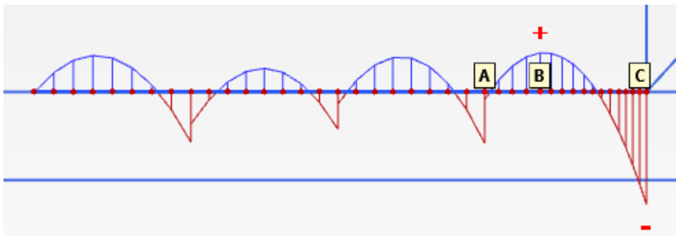
Figure 3. 27. Critical sections at bottom slab
