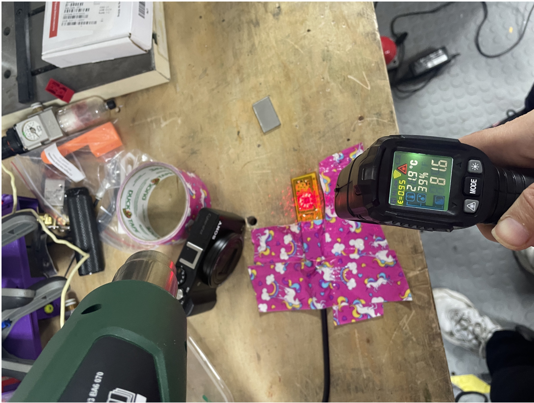
Figure 7.5: Heating Attack on TRNG OneRNG device
