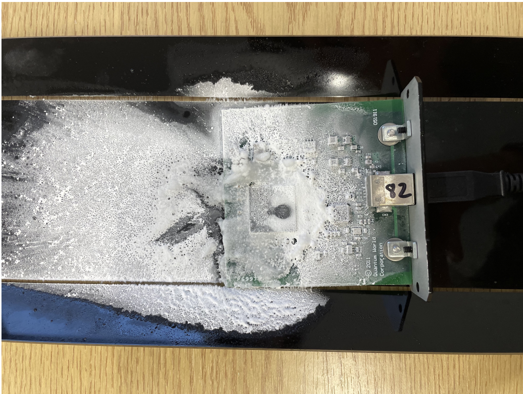
Figure 7.2: ComScire device after Cooling experiment
