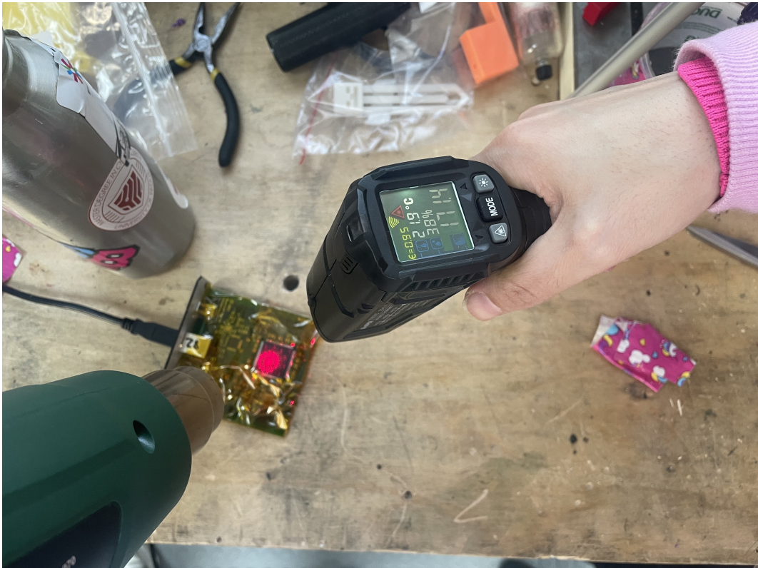
Figure 7.6: Heating Attack on QRNG ComScire device
