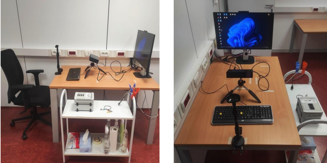
Figure 8. These photos were taken from the experimental setup (a lateral view on the left and a frontal view on the right). The sequence includes the adjustable chair, the chin-rest, the keyboard, the tripod equipped with the eye-tracking device and the monitor presenting the experimental conditions. On the side, the amplifier to which the hd-EEG is connected, is placed on a trolley.
