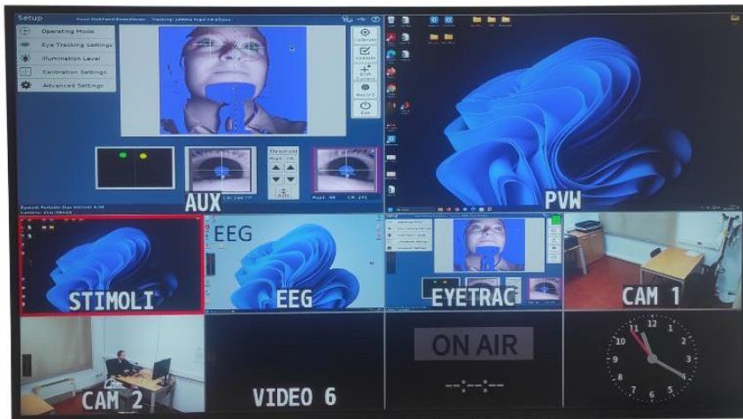
Figure 9. Shown in the photo are the monitors located in the experimenter’s room: the stimuli presentation PC, the EEG system, the eye-tracker device interface and the feeds from two cameras used to monitor the participant.
