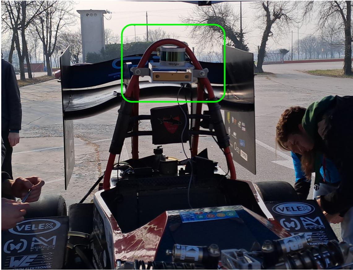
Figure 5.5: Sensors support mounted on the main hoop
