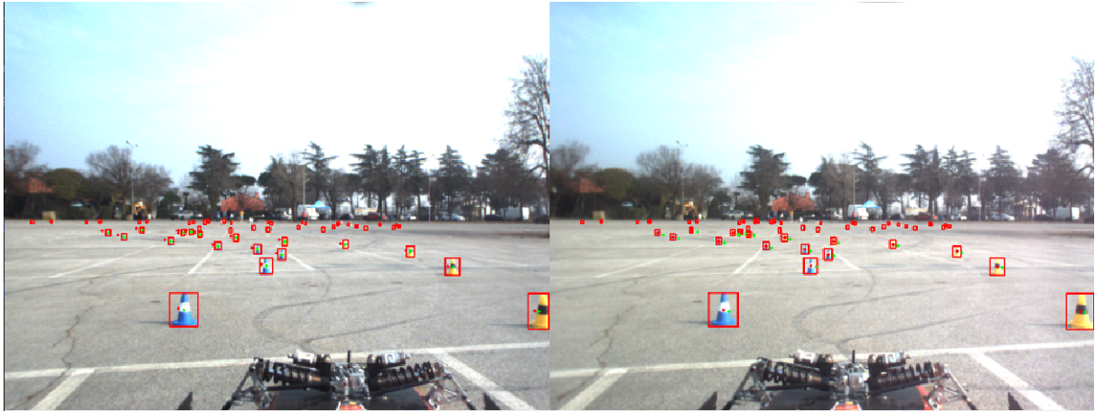
Figure 6.4: Green dots are centers estimated in the left image and red dots are centers estimated in the right image.
