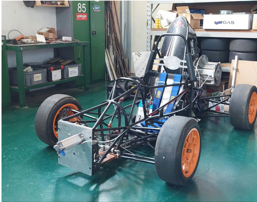
Figure 4.3: RaceUp MG03, modified to be the test mule
