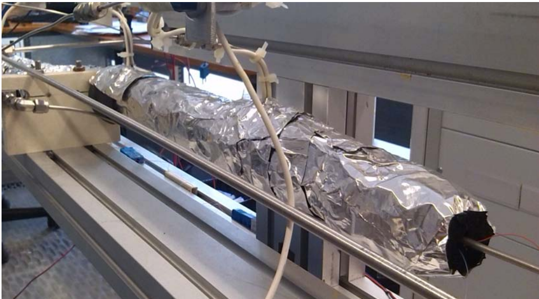
Figure 4.6: Picture of the pressure drop test section installed in the test rig.
