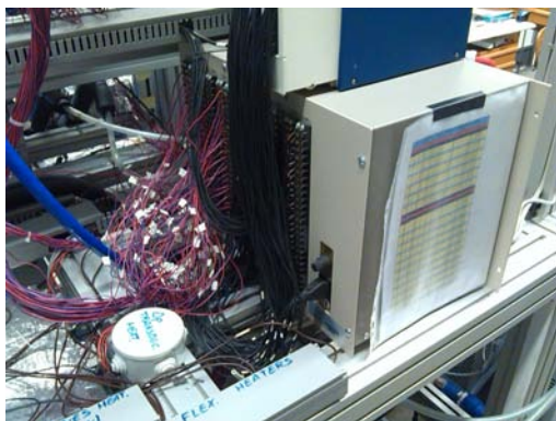
(a) Kaye instrument, reference for 0^{\circ}\text{C} .
