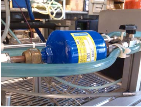
(a) Mechanical filter and a dehumidifier.
