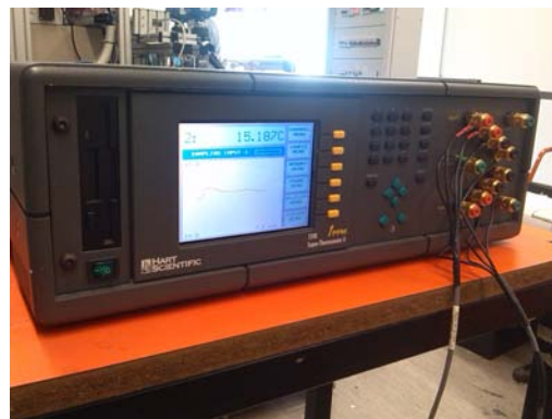
(b) Super thermometer for thermocouples calibration.
