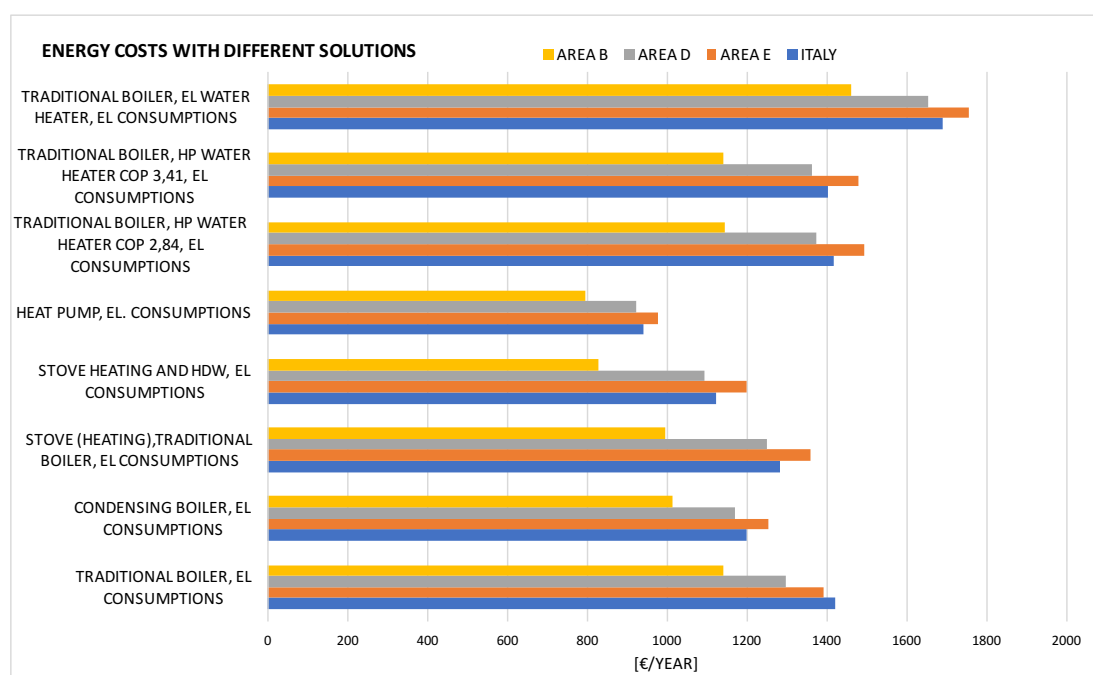
Figure 37. Energy costs of diverse solutions (without considering the investment cost of this installations).
