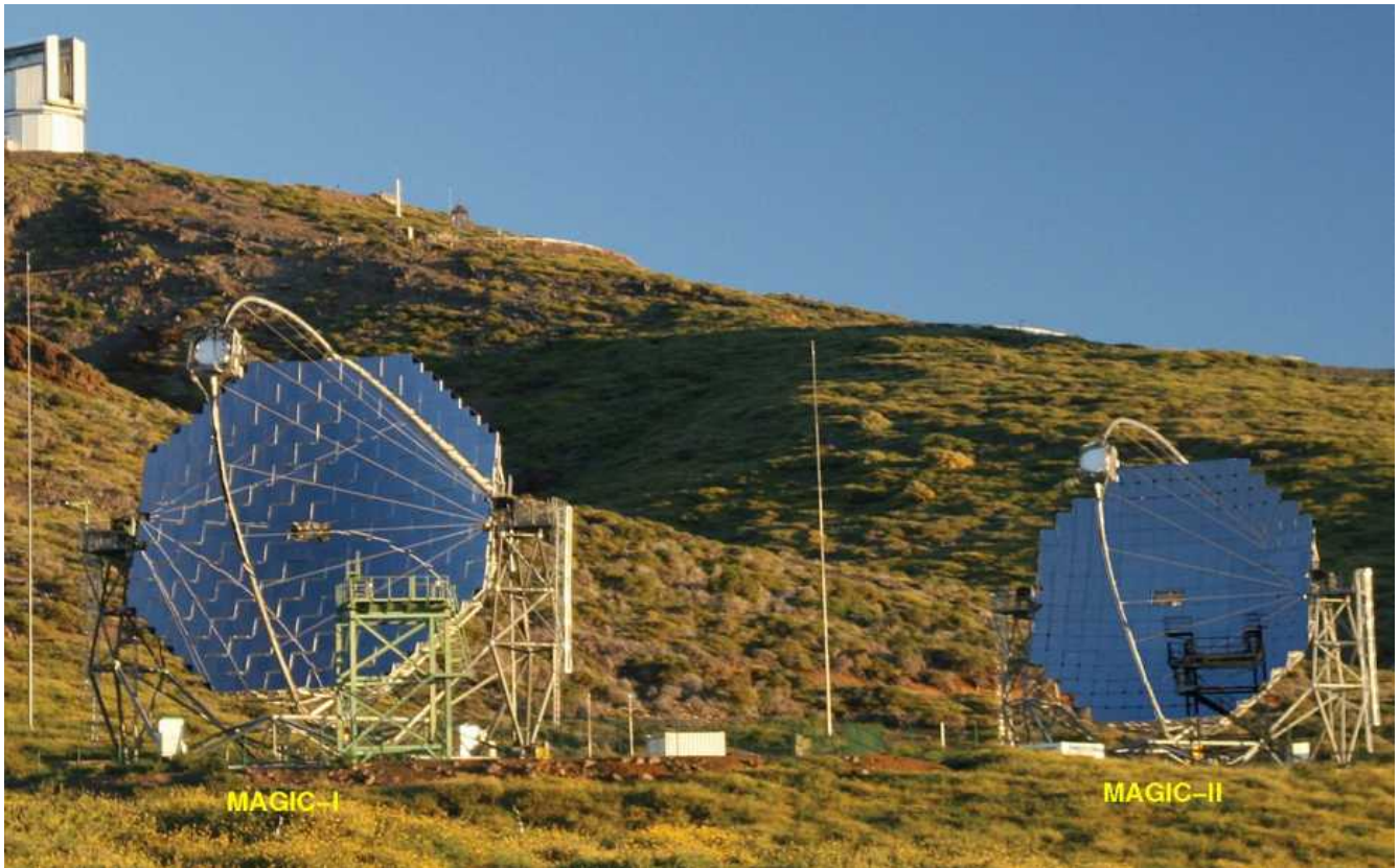
Figure 3.3: MAGIC telescopes, Roque de los Muchachos Observatory. On the left side MAGIC-I is active since 2004, on the right side MAGIC-II is active since 2009 to significantly increase the sensitivity by stereo observations. MAGIC are the largest of the current Cherenkov telescope systems. Both instruments are made up of individual mirror panels that can be independently focused using an active mirror control system equipped with lasers.
