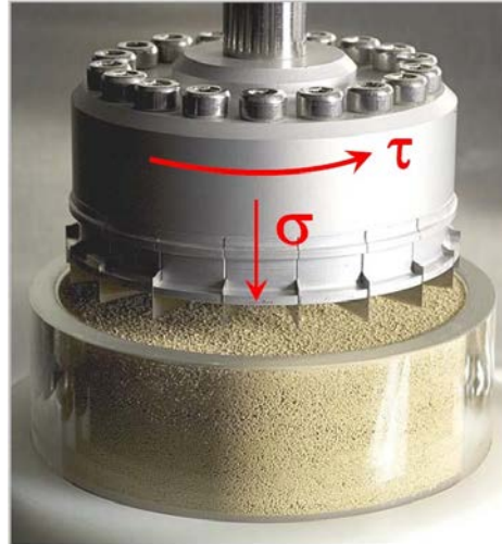
Figure 2.11. Rotation Shear cell of the FT4 powder rheometer (Freeman Technology, W7018, 2010).
