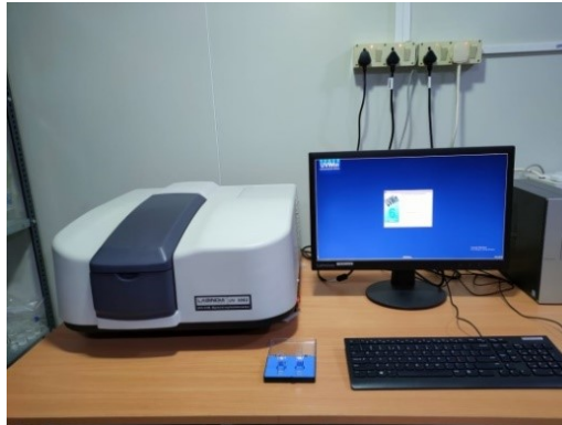
Figure 2.5: Lab India Spectrophotometer.
