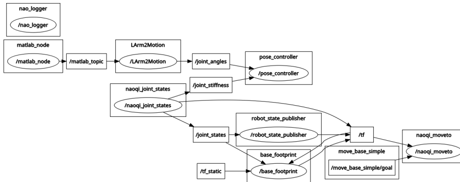
Figure 4.5: rqt_graph GUI plugin display of the ROS network created for the NAO robot control
