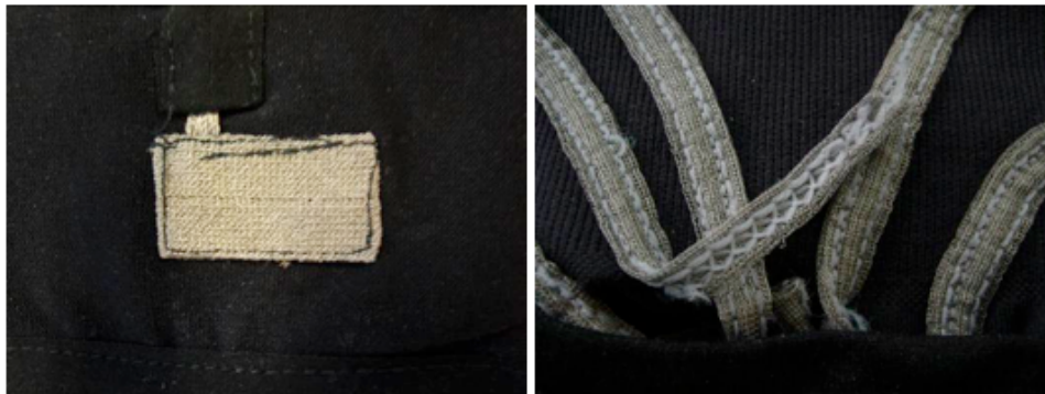
Figure 2.4: Silver ECG electrode (left) and silver wires (right) used to conduct the ECG signal inside the T-Shirt.
