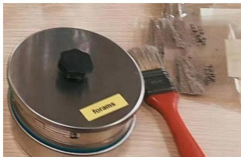
Figure 5.3.1: the 128\mu\text{m} aperture sieve (left) and the coarse brush (right) used.
