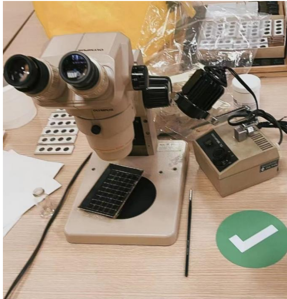
Figure 5.3.2: the optical microscope (middle), the plate with reference grids (under the microscope), the fine brush used (right side of the microscope), the bottle of deionized water (left side of the microscope) and the sealed sample holders (top left).
