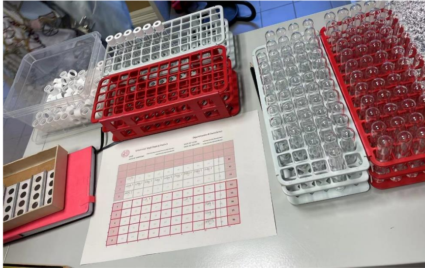
Figure 6.2.2: 10-ml round-bottomed borosilicate exetainers (right) and the butyl rubber septa (top left).
