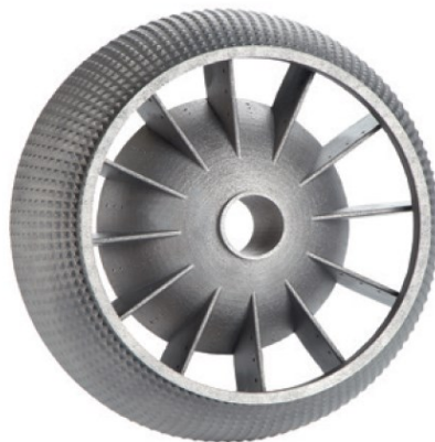
Figure 2.4. Air duct manufactured with PBF (diameter = 20 mm ) [35]
