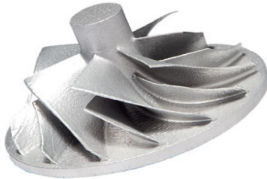
Figure 2.5. Pump impeller manufactured with PBF (diameter = 17 mm) [35]
