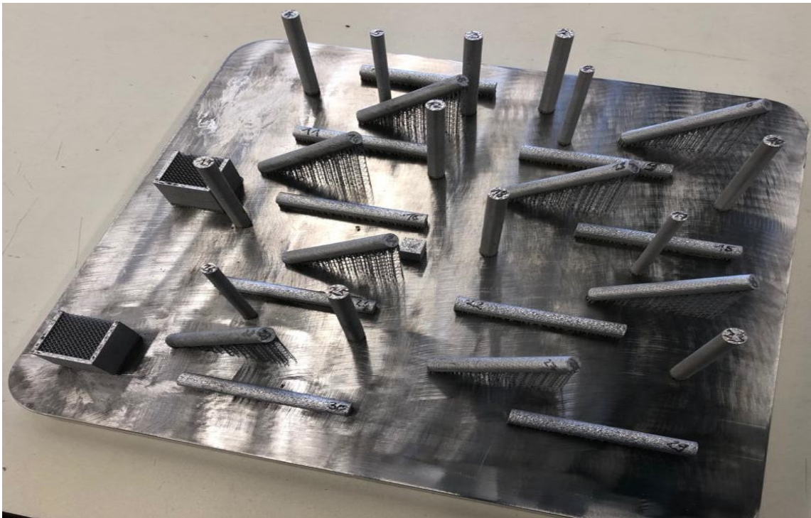
Figure 4.3. Compression cylinders arrangement in the machine table
