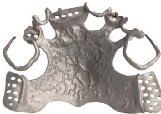
Figure 2.6. Dental plant manufactured with PBF (8 mm x 6 mm) [35]
