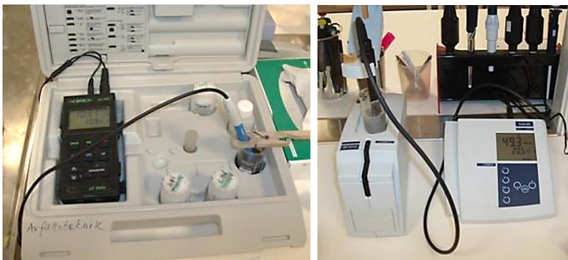
Figure 4 (II). The pH-meter and EC-meter were used to evaluate pH and EC right after the sampling. The values calculated are summarized in Table 1 at the end of the thesis.
