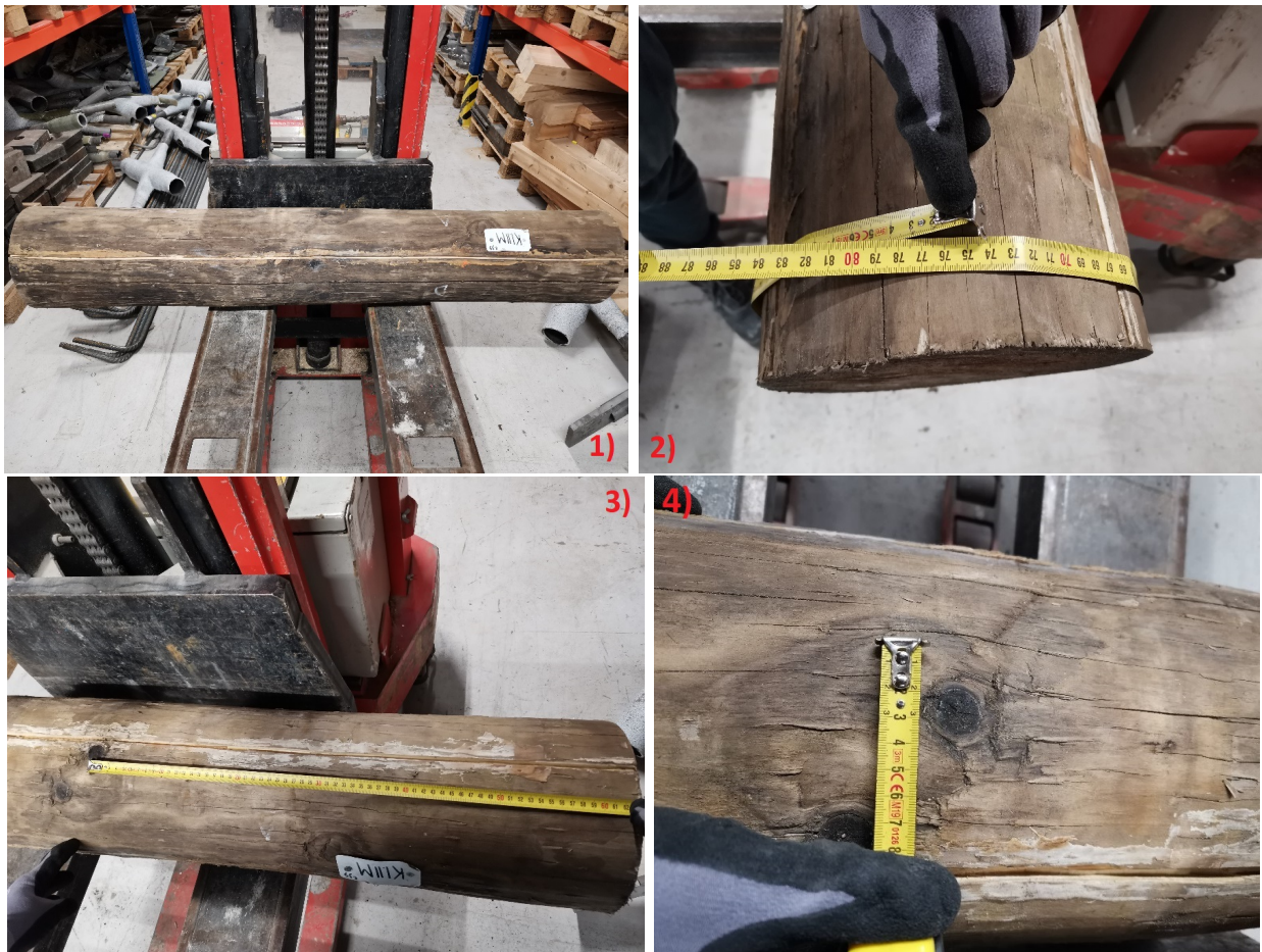
Figure 5.1.3: 1)Preparation of the sample; 2)Identification of the sample head; 3)Position of the knot; 4)Knot size measurement.
