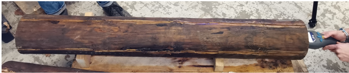
Figure 5.2.5: MTG measurement of the dynamic response of a pile;
