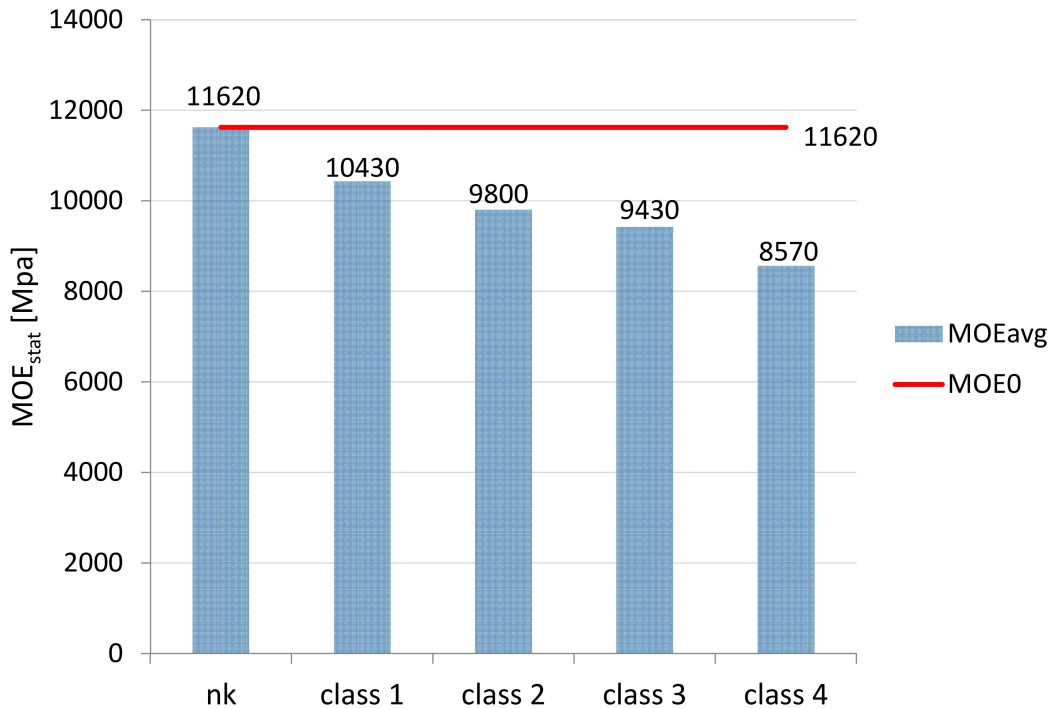
Figure 7.1.3: variation on the MOE for each class of piles with different values of OKR_A ;
