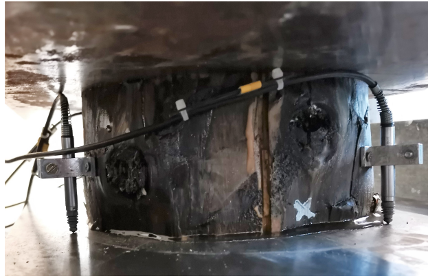
Figure 6.3.3: example of a compression test on disks M1.1V with knots;
