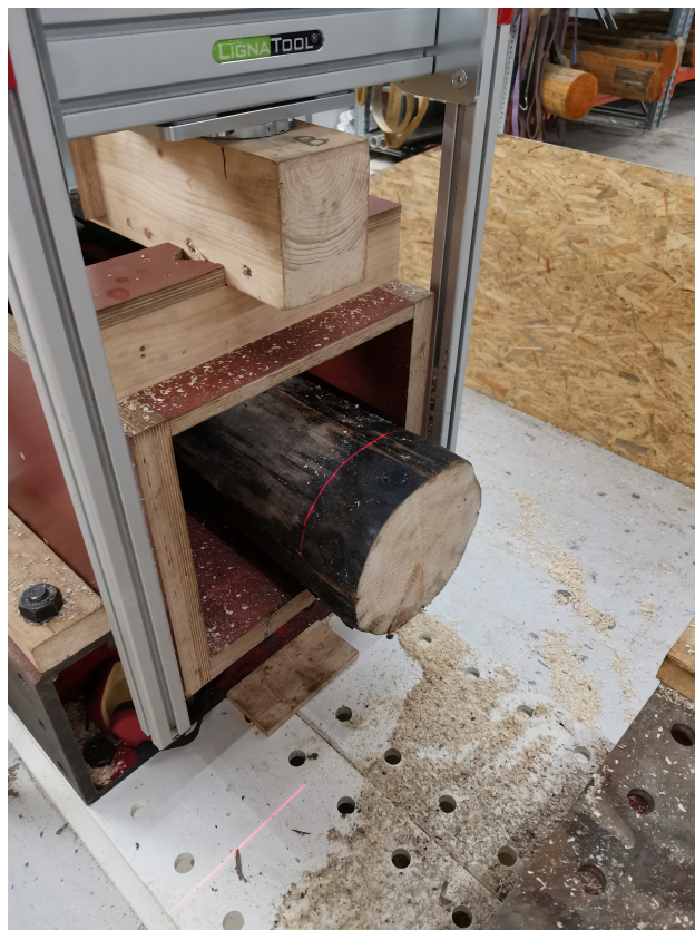
Figure 4.0.6: cutting procedure of the pile M1.1V;
