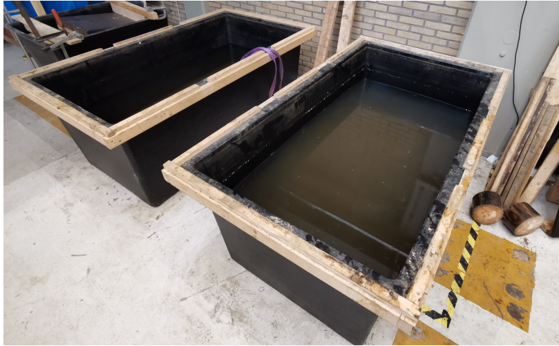
Figure 4.0.3: tank filled of water, at TU Delft laboratory, to dive piles under water ;
