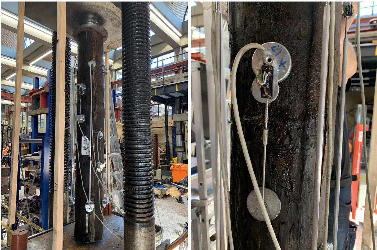
Figure 5.2.2: example of uniaxial compression test on a pile on the right and the position of a linear potentiometers around a knot area on the left;
