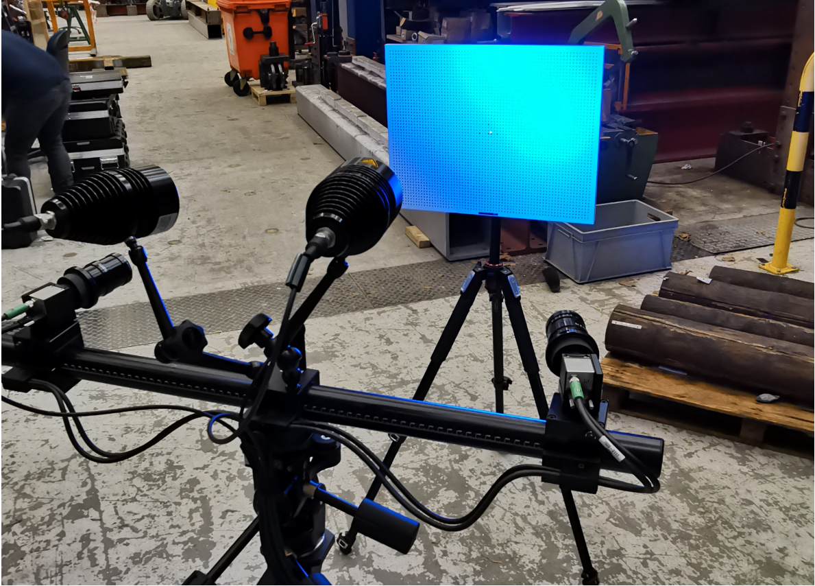
Figure 5.3.8: DIC cameras calibration;
