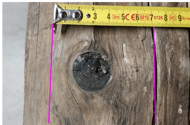
Figure 5.1.2: example of knot measurement taking into account the inclination of the fibers;
