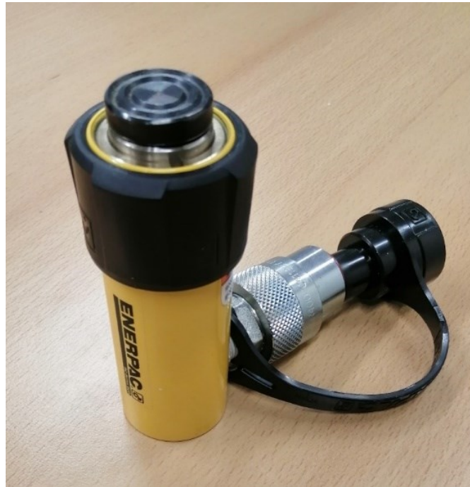
Figure 4.7 The RC51 hydraulic cylinder used in the calibration.
