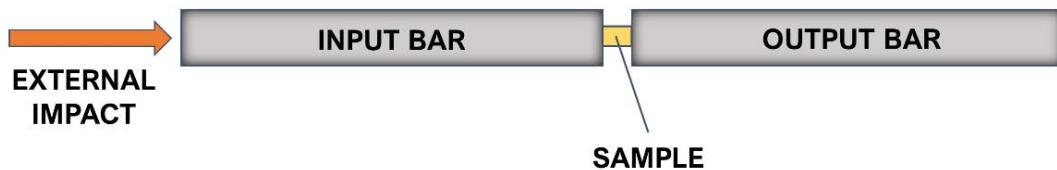
Figure 3.1 Schematic representation of the Hopkinson Bar loaded in compression.
