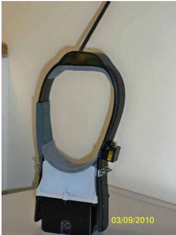
Figure 1.4 GPS camera collar unit (Thompson et al., 2012)
