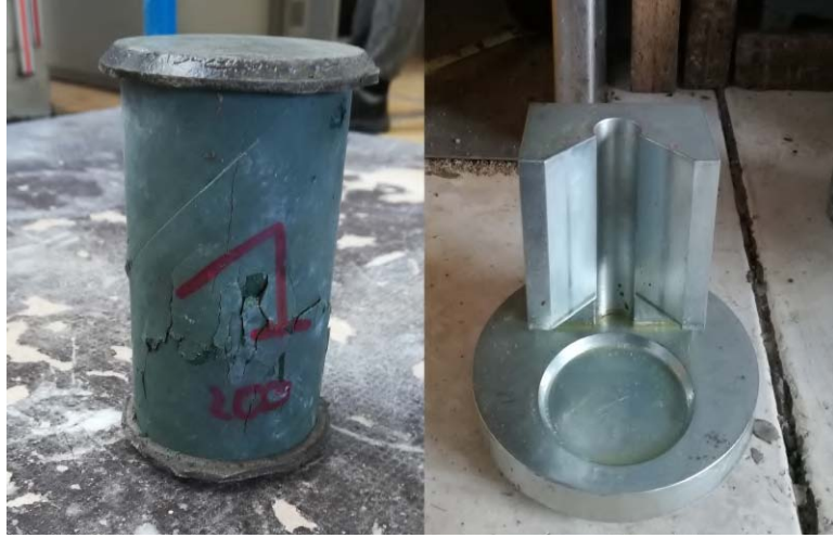
Figure 2.10: Equipment employed in surfacing with sulfur
