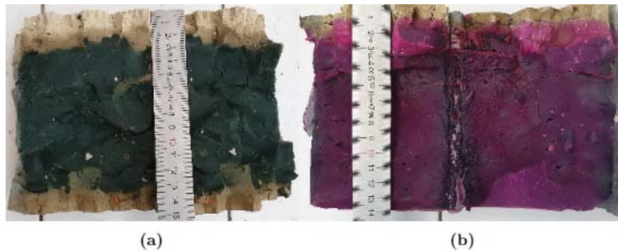
Figure 3.18: Measure of (a) internal drying and (b) carbonation depth
