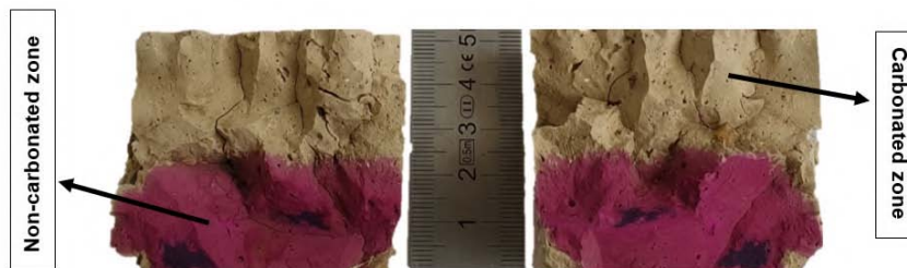
Figure 3.17: Carbonation depth of a soil-cement specimen subjected to a relative humidity of 65%
