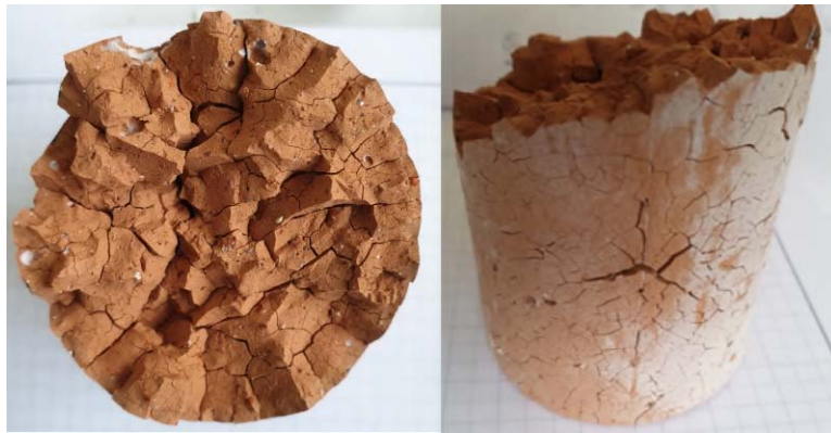
Figure 3.40: Specimens after 850 °C
