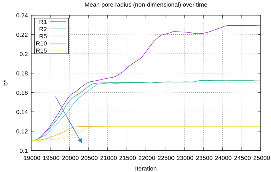
Figure 5.14: Comparison of the distribution of the non-dimensional mean pore radius (for configuration R1,R2,R5,R10 and R15) over time. Arrows points in direction of increasing energy release rate.
