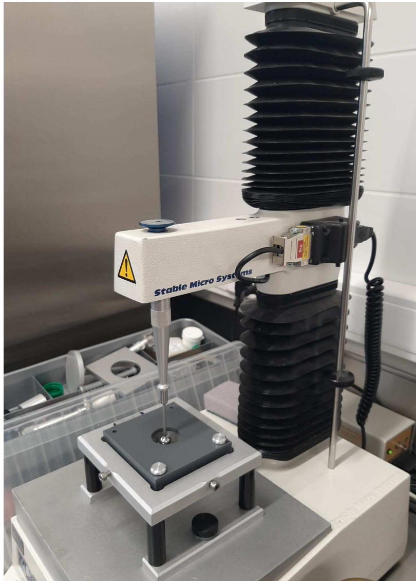
Figure 13: SMS Tensile Strength (Puncture test) Machinery and the platform that is designed to hold the films
