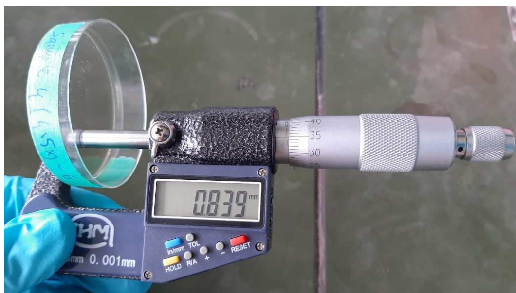
Figure 29: Measurement of the thickness of the film with a micrometre
