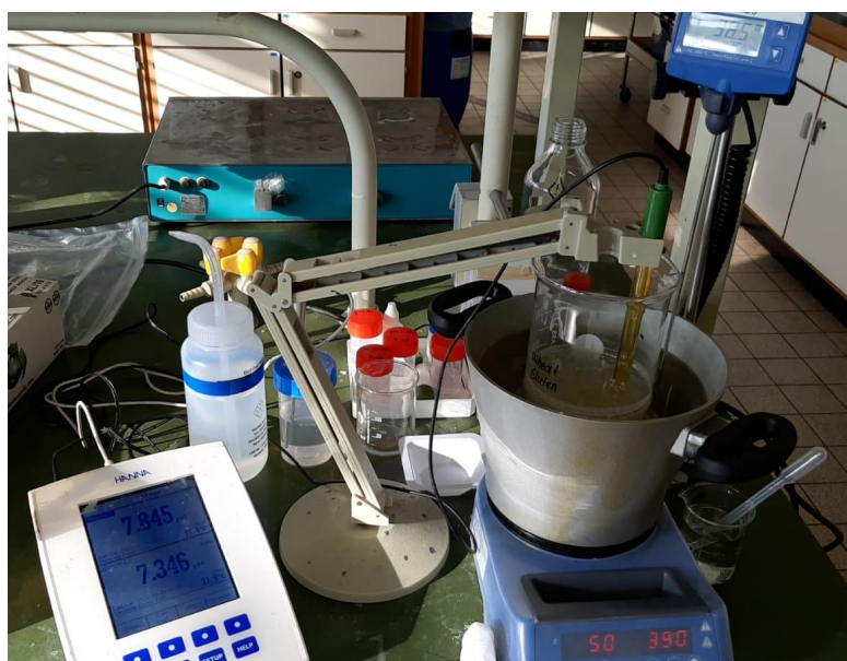
Figure 8: The experimental setup for hydrolyzation of wheat gluten
