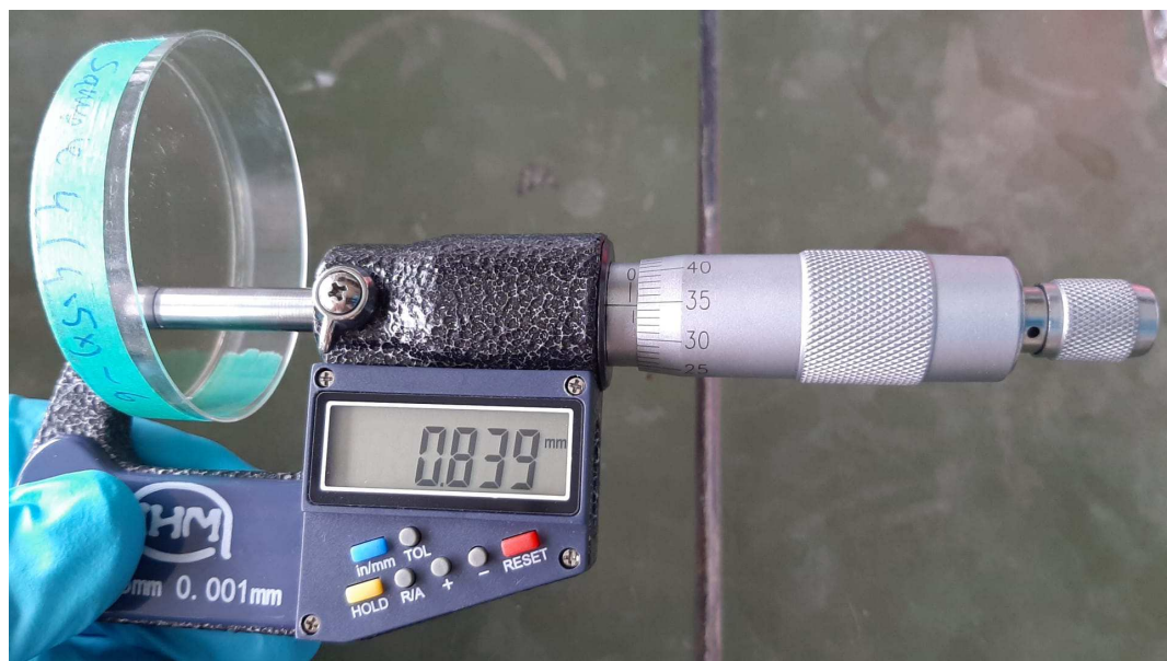
Figure 15: Measuring the thickness of the films with a micrometre
