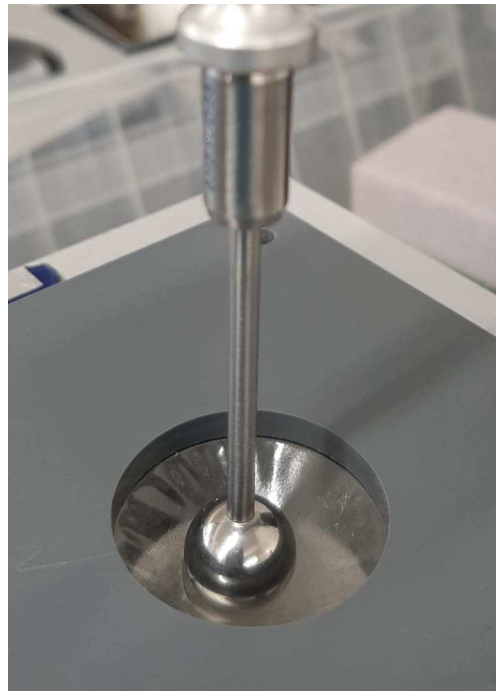
Figure 14: Probe pushing through the film
