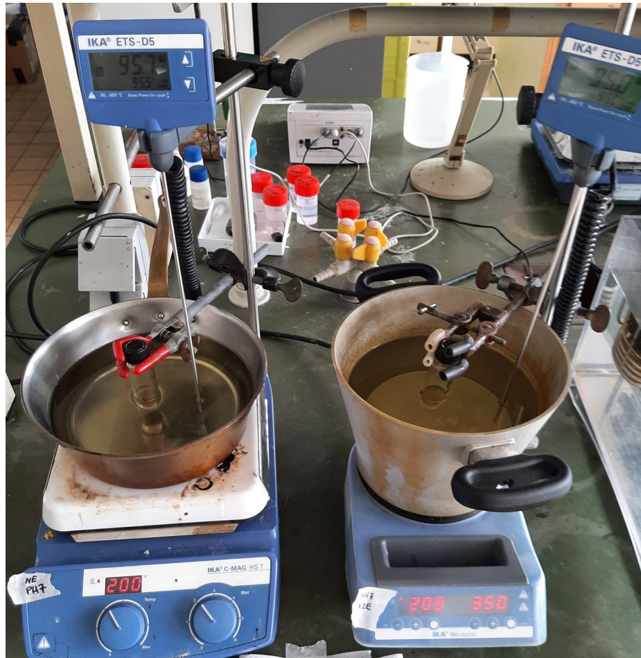
Figure 11: Experimental setup for the incubation of the wheat gluten protein samples
