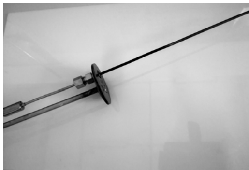
Figura 3.5: Termocoppia (TC) Multipoint.
