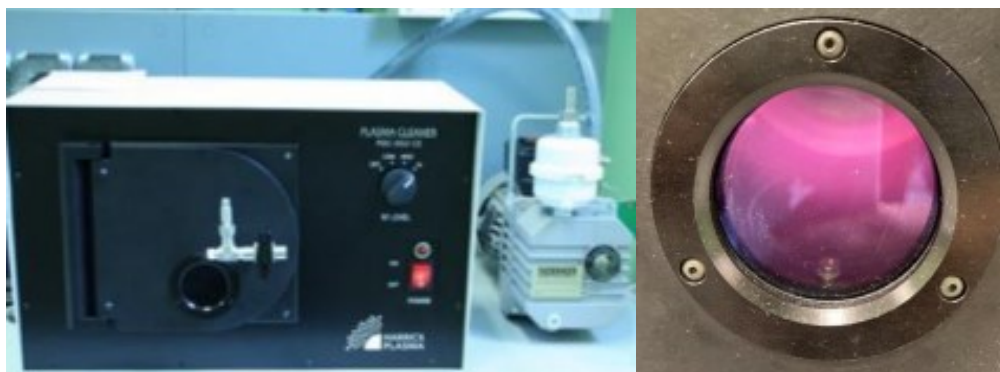
Figure 2.7 (a) Plasma cleaner and (b) the color of the plasma inside the chamber in the right configuration.
