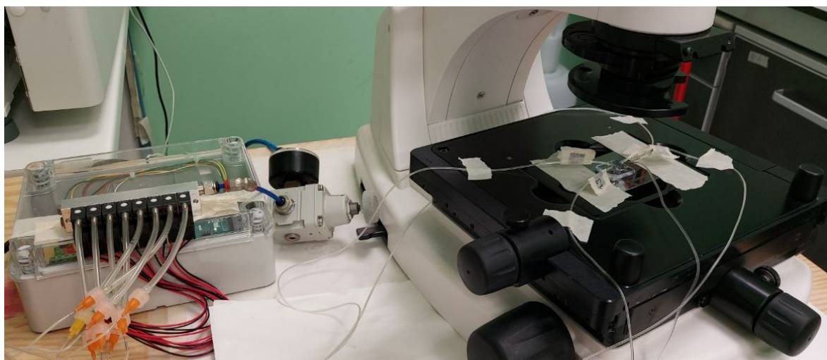
Figure 2.12 Overview of solenoid valves connected to microfluidic platform.
