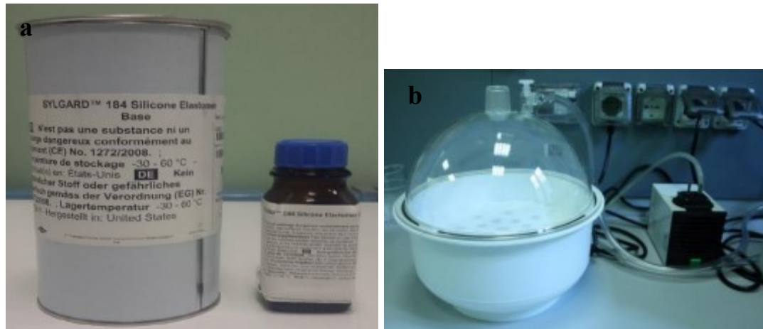
Figure 2.8 (a) PDMS Sylgard® 184 (Dow Corning), two-part kit: silicone elastomer base on the left, curing agent on the right. (b) Desiccator connected to a vacuum pump.
