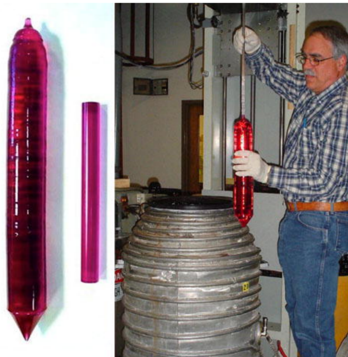
FIGURE 3.2 • A Czochralski-grown synthetic ruby crystal with a fabricated piece (left) and during extraction (right). Photos by Jennifer Stone-Sundberg [59].
