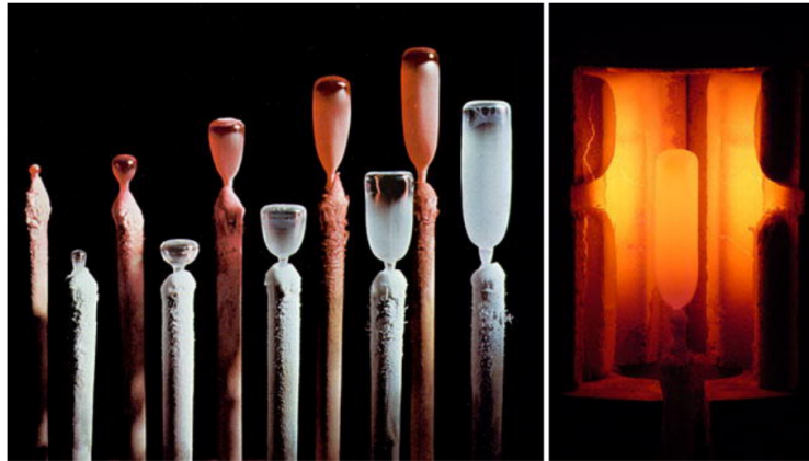
FIGURE 3.1 • Flame-fusion synthetic sapphire crystals, as-grown (left) and during growth (right). Courtesy of Hrand Djevahirdjian, SA [59].
