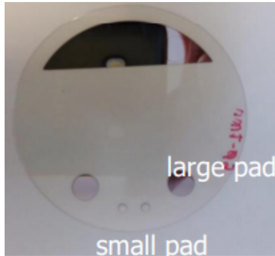
FIGURE 5.1 • Sapphire pads tested at INFN-Frascati.
