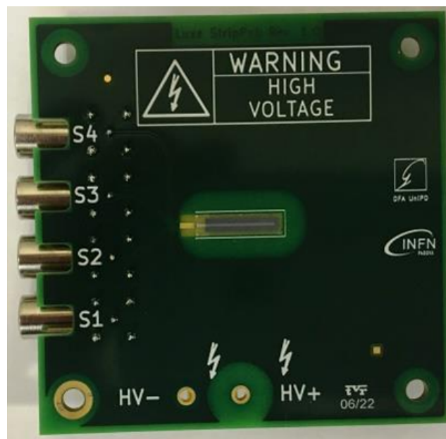
FIGURE 5.2 • The Sapphire 4-strip sensor that was tested at CLEAR (CERN).
