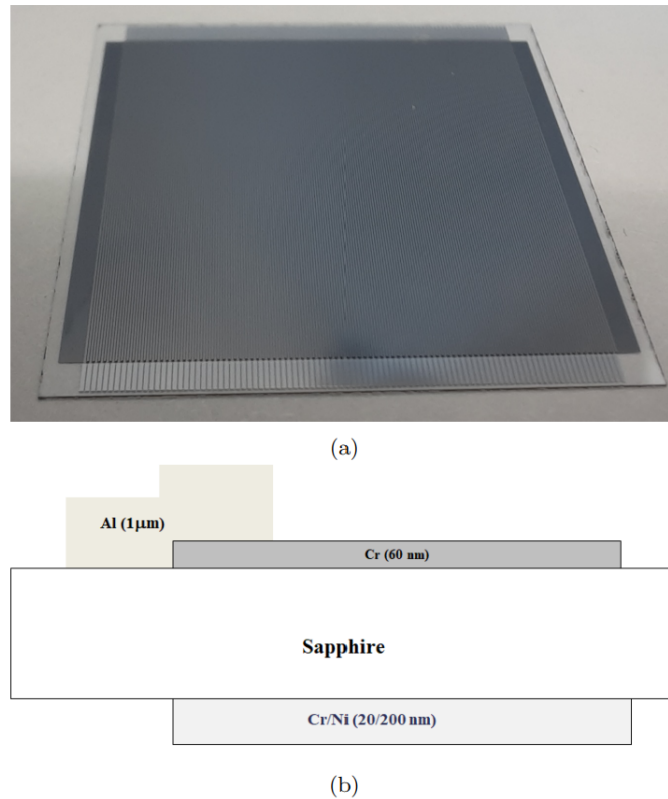
FIGURE 5.4 • (a) A close up perspective of the 192 microstrips sensor. (b) Sensor contact structure [3]
