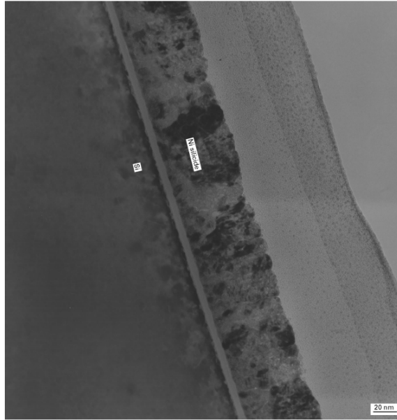
Figure 3.4: Formation of nichel-silicide after annealing treatment; as we can see from the picture the structure of the barrier is still intact and the presence of the silicide does not affect the effectiveness of the barrier[15]
