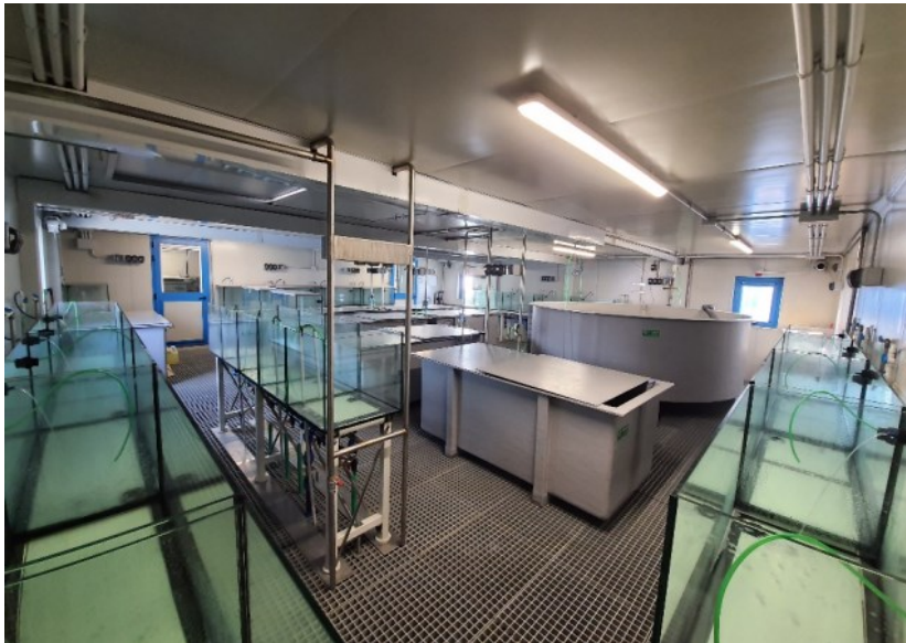
Figure 3.3: The aquarium laboratory at the Mario Zucchelli station, inaugurated during the 2020-2021 campaign. The infrastructure consists of a series of tanks of different volumes, which can also be used individually, in which it is possible to adjust the temperature and dissolved gases, and continuously monitor the pH, dissolved oxygen, conductivity and temperature values (PNRA).
